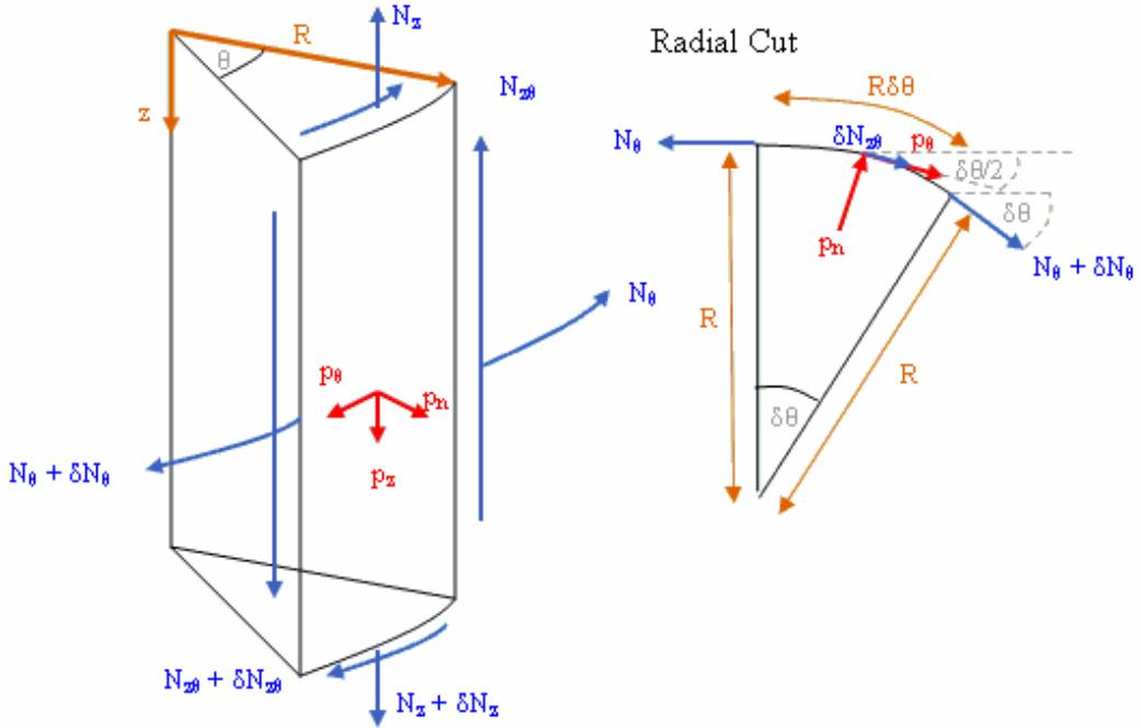
Use small angle approximation: As  $\partial\theta \rightarrow 0$ ,  $\cos\partial\theta \rightarrow 1$  and  $\sin\partial\theta \rightarrow \partial\theta$ , and also  $\partial\theta^2 \approx 0$ ,  $\partial N_\theta \approx 0$ .
